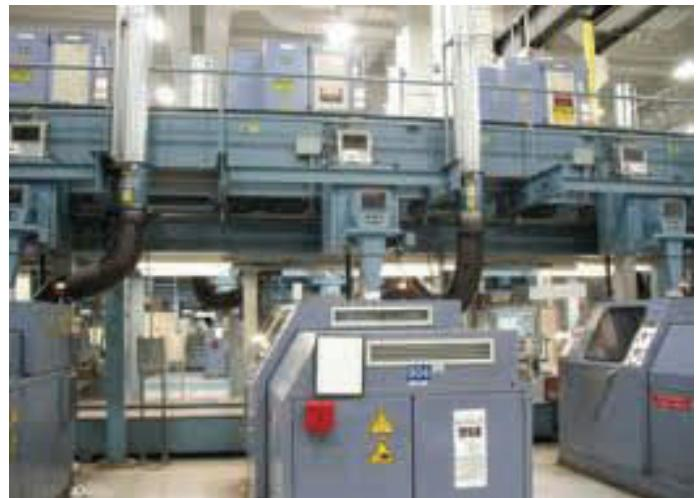
Finally, they were transferred to rows of minting machines like the one in the photo above. Afterward they go into huge bins, where they are taken to be put in bags for distribution. The bags are about 2' cubes, and the coins are counted by weight, not by the exact number.
