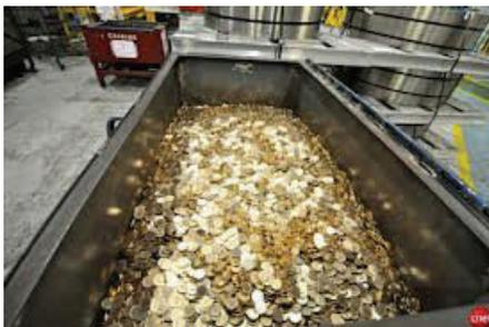
Planchets went through annealing to heat them up and soften them for easier pressing, seen in this photo. Then they were washed, dried, and an edge rolled onto them.
